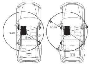
The sound is not balanced because the distance between the listening position and the various speakers is different. The difference in distance between the front left speaker and the rear right speaker is 1.75 m (68-7/8").
